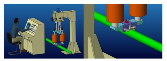
Eddy Current Testing System for High Frequency Electrical Resistance Weld
