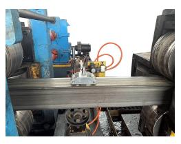
Weld Seam Inspection of Square Tube
