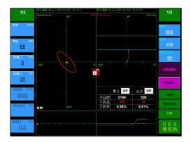
The two-channel instrument is used to drive the differential and absolute probes respectively, and the holes, inclusions, cracks, leakage welding and long-distance open tubes of the welded steel pipe are detected. When defective products are produced, it will timely report the alarm, output the bad alarm signal and mark, and defective products sorting signals are sent to the sawing control system of the unit.
